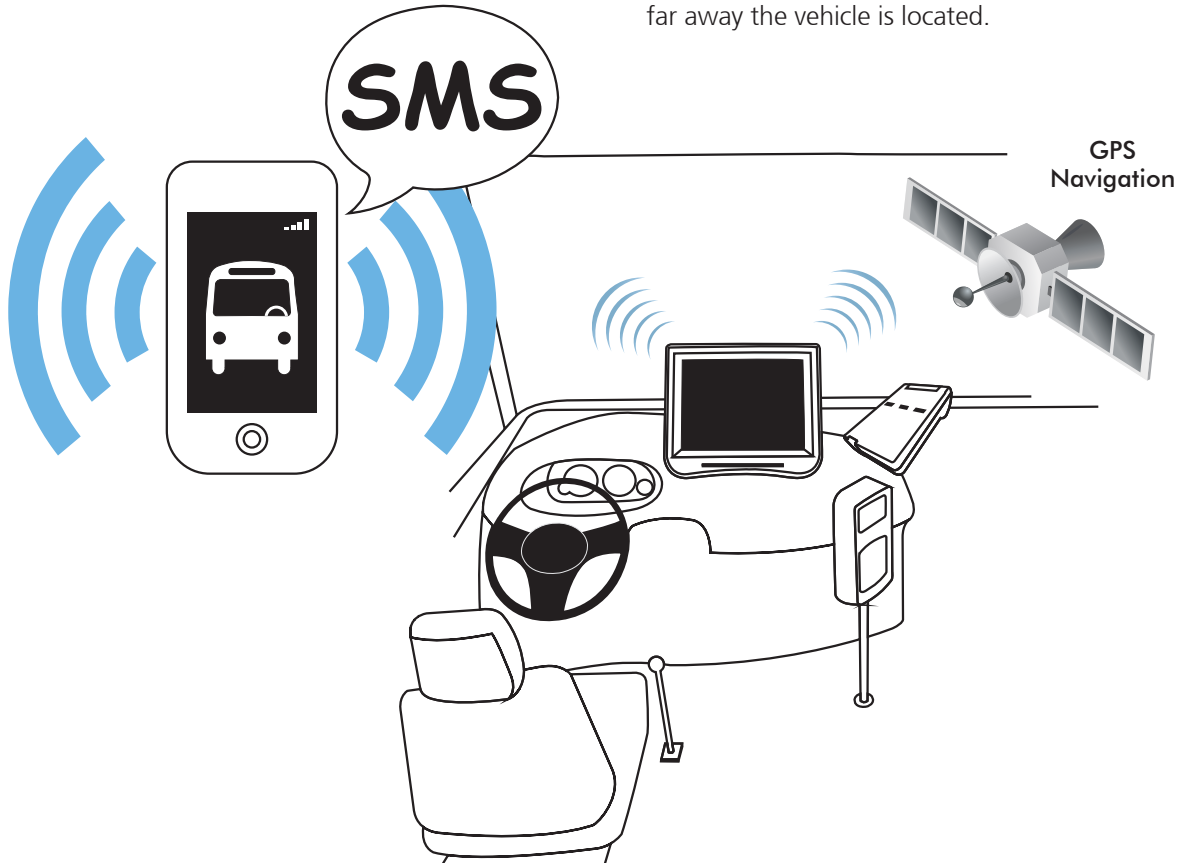
Figure 1. With integrated wireless network modem, the VTC 1000 in-vehicle computer can be activated by remote wake-up feature using SMS.
